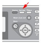
2 Press the down arrow key to select [Paper Setup], then press <OK>.
