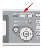
2 Press the down arrow key repetitively to select [Shutdown]. Press <OK>.
