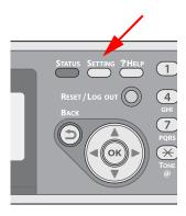
Press the down arrow key repetitively to scroll to [Admin Setup], then press <OK>.
